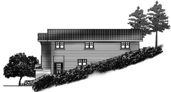
Building forms do not step down with the existing grade.
