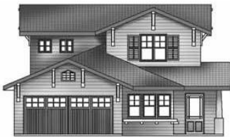
This second story addition centered over the lower floor away from property lines appears less boxy.
