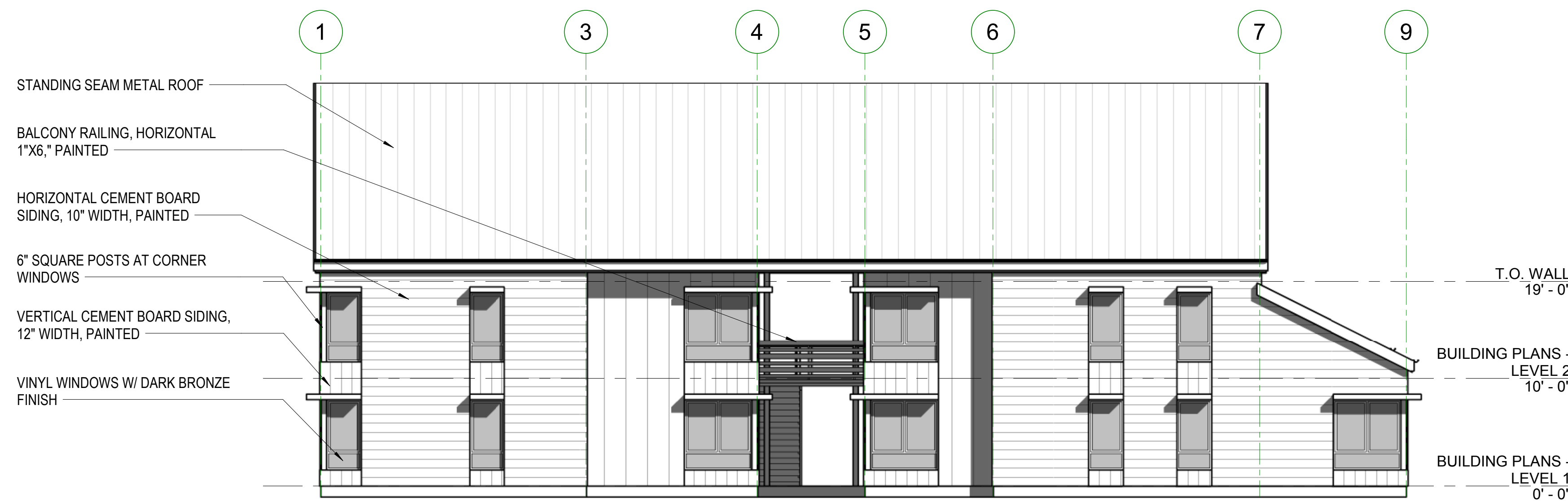
BLDG TYPE C - SOUTH ELEVATION 1/8" = 1'-0" 5
