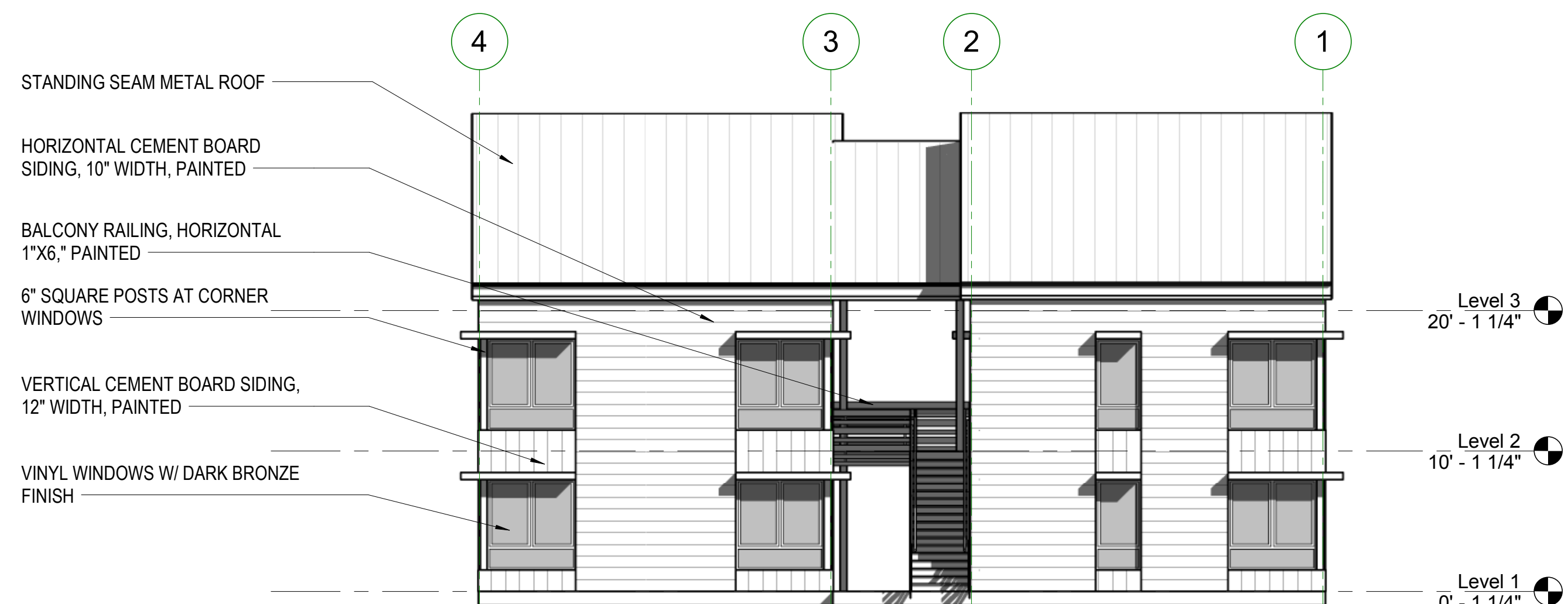
BLDG TYPE B - SOUTH ELEVATION 1/8" = 1'-0" 5
