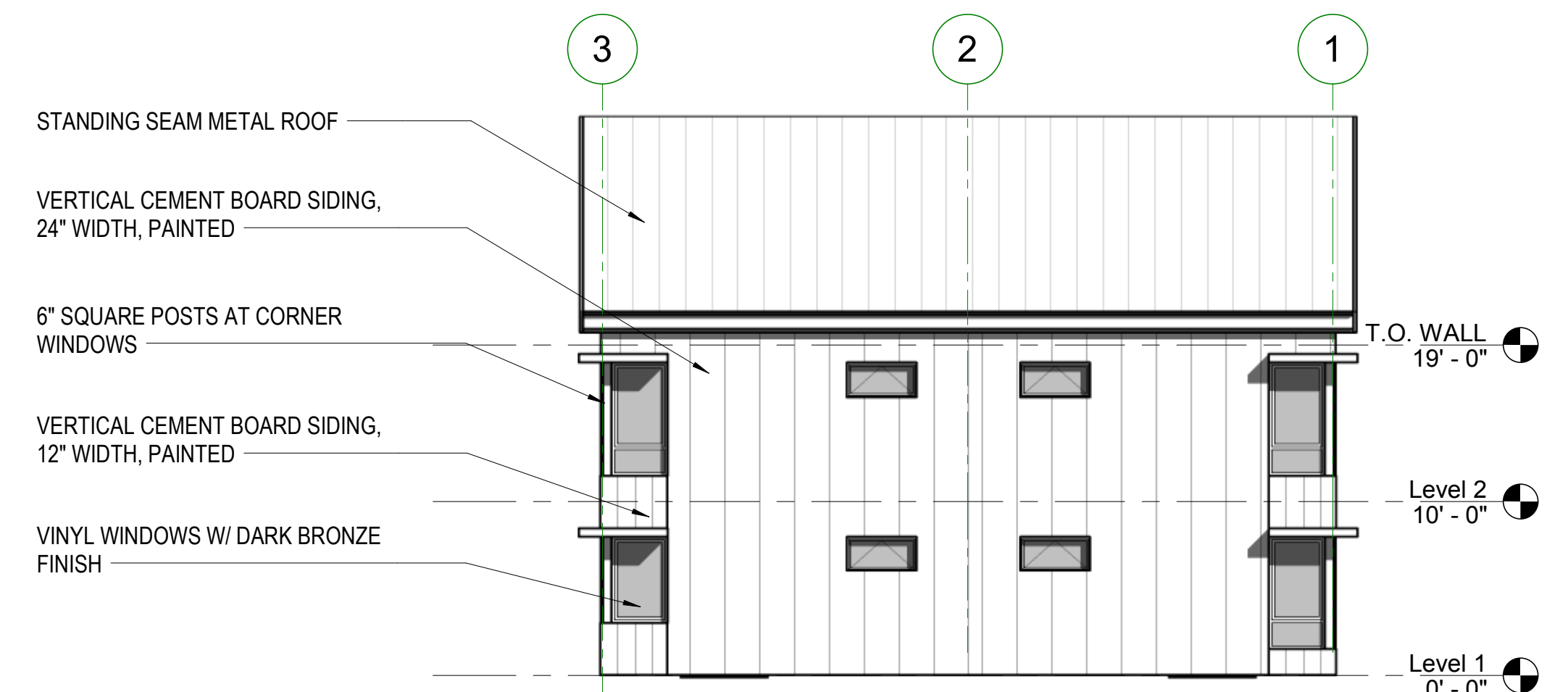
BLDG TYPE A - NORTH ELEVATION 1/8" = 1'-0" 4
