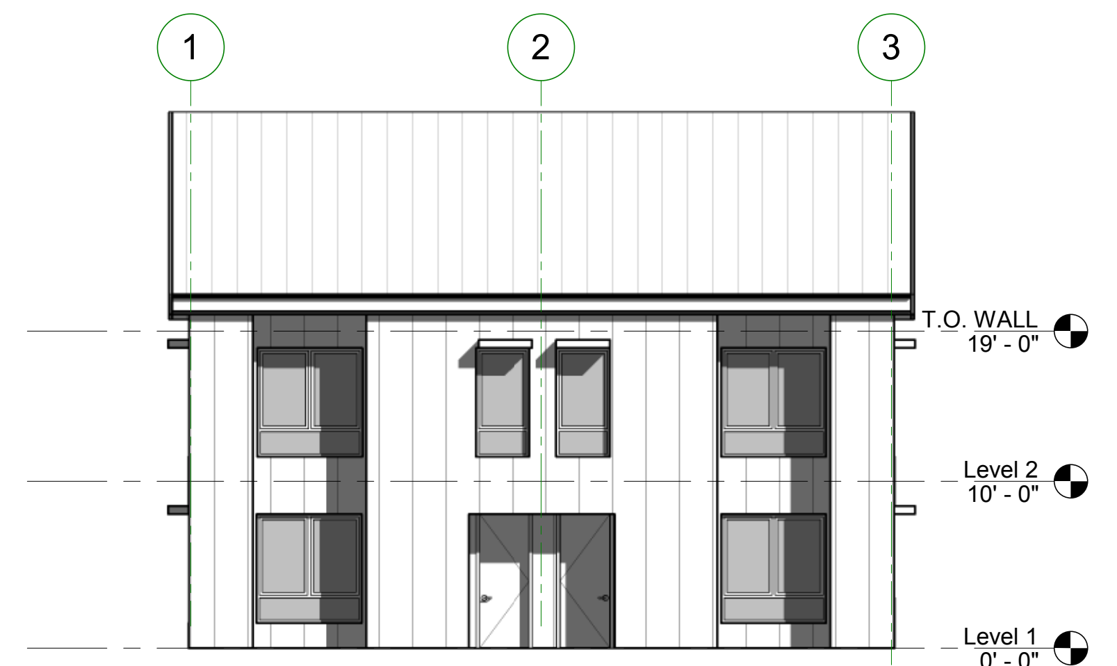
BLDG TYPE A - SOUTH ELEVATION 1/8" = 1'-0" 5
