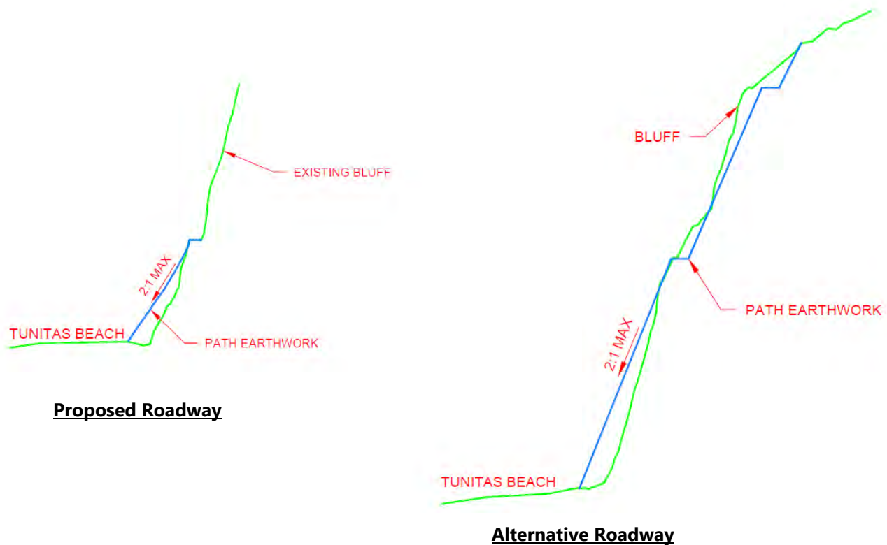
Figure 6. Proposed and alternative access roadway typical sections.
