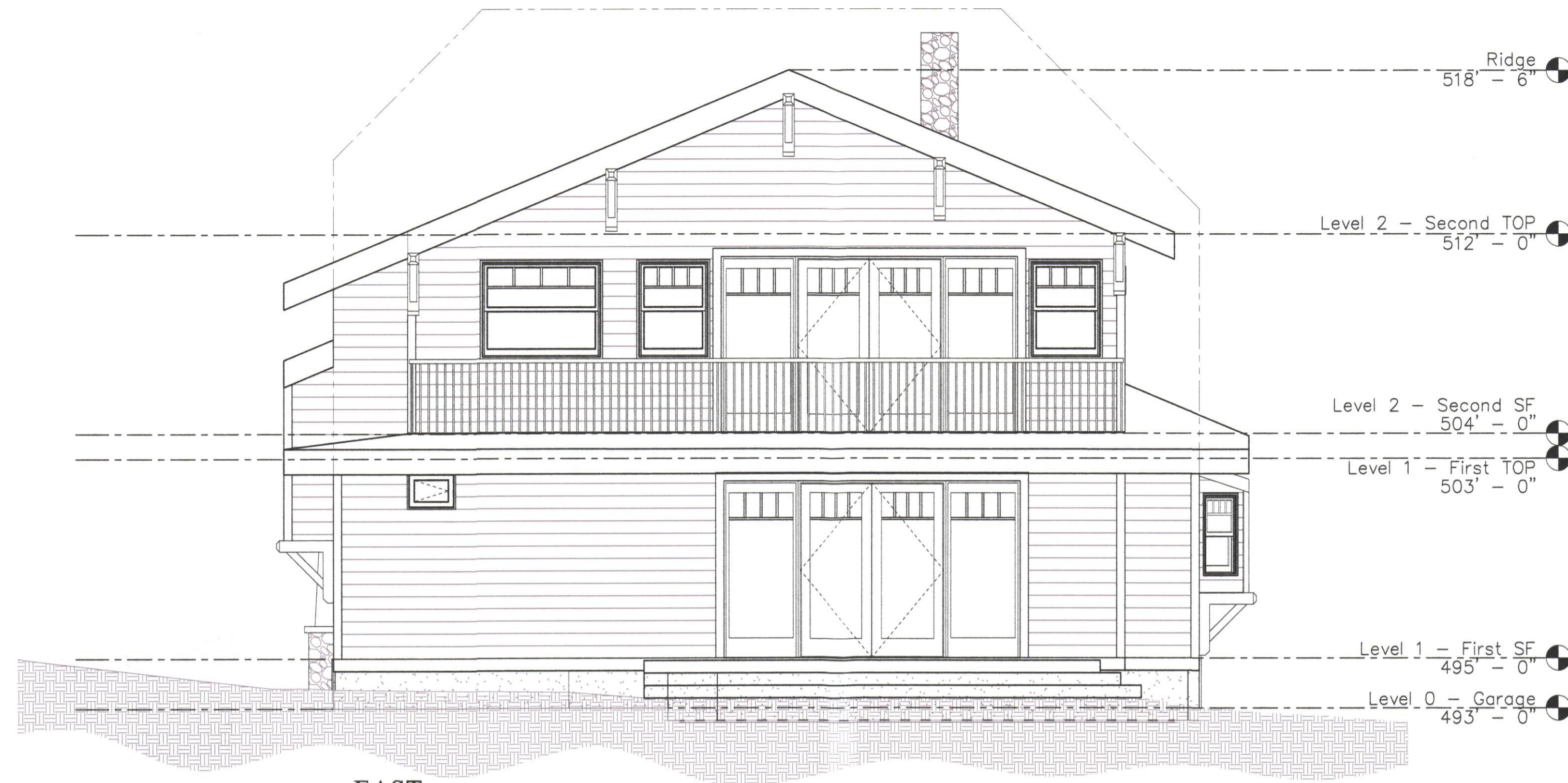
3 A4.2 EAST ELEVATION (BACK)
